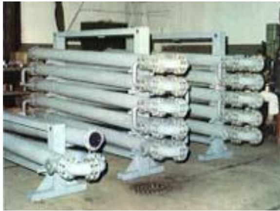
Jacketed Pipe Heat Exchanger- keeps reactions at proper temps
