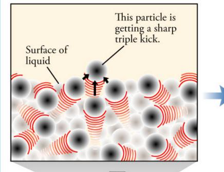
The kick propels the particle out of liquid.
