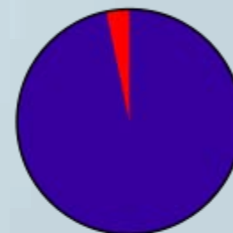
Low-enriched uranium (reactor grade) 3-4% U-235
